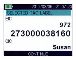
If the option is set, a dialog requesting a tag labels is presented after a tag is read. Tag labels can also be edited as a text file and re-imported to the reader using SoftPC.
