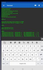
A nice setup is an Android tablet with a waterproof case running Kai's Serial Bluetooth Terminal. Capture files can be stored on the tablet and emailed or uploaded to a cloud service.
