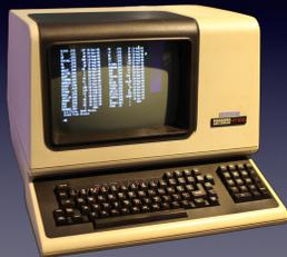
In olden times, the human interface to a computer was a mechanical terminal connected by a serial cable. Characters were typed on a keyboard and the computer's response was printed on paper. Terminals using video screens of scrolling text eventually replaced them.
